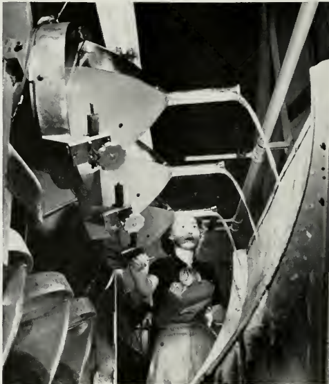
At the terminal of the "settling belt," the water of the phosphor solution pours out into a spillway, leaving a fluorescent coating on the faceplate.
