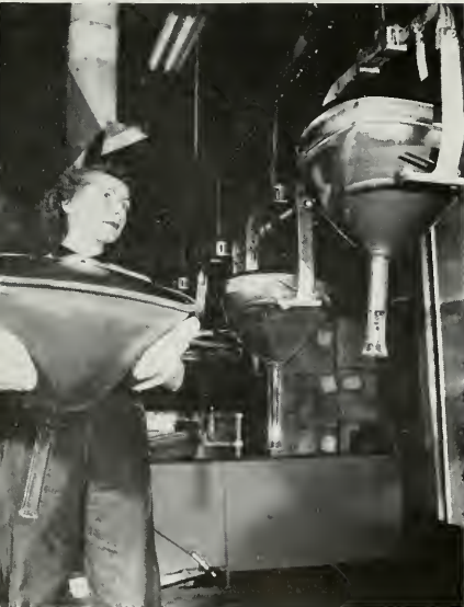
Some of RCA's employees at the Lancaster plant load metal-shell picture tubes on the overhead conveyor system.
