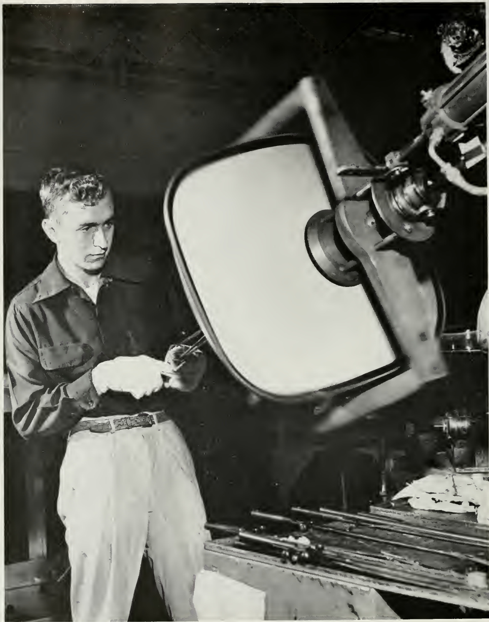
In making a picture tube for a television receiver, the kinescope is whirled rapidly while a graphite coating is applied to the inside of the glass neck and metal cone at the RCA plant, Lancaster, Penn.
